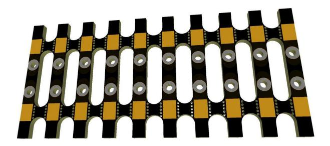
The JTETT1-HO track tie / power feeders can be used to simply and reliable connect power feeder wires to HO scale track. Since the JTETT1-HO is soldered to the track rails, it will also keep the track rails at the correct spacing. You can also snap off two adjacent track tie boards to join the ends of two blocks of track and provide power connections to both track blocks.
