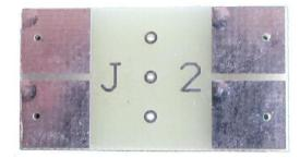
The JTETJ2 track rail joiner can be used to simply and reliably join HO scale flextrack by soldering the JTETJ2 track joiner to the track rails as shown in the photos below. You just remove a few plastic "sleepers" from the ends of the flextracks to be joined, slide the JTETJ2 board under the tracks and solder the <u>outside</u> of the track rails to the JTETJ2 track joiner.
