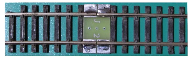
This image shows the top track rail has been cut, maybe with the likes of a Dremel tool, <u>after</u> the track joiner was soldered in place. The cut ends of the track are still perfectly aligned so there is little chance of a derail... Russ can now easily solder one of my block detection sensors between the two top terminals.
