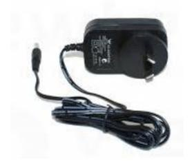
For HO scale use I have seen good results with using an old Toshiba laptop charger like in the picture to the right, and these are usually rated for 15V DC at 5Amps. You will need to carefully check the label to make sure it's rated at 15V DC as some laptop chargers are 18V or 19V DC and this will be too high! ie. Will damage the DCC Decoder and/or motor in the locomotive!
