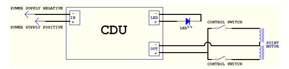
The diagram shows a single point motor being operated but you can connect two point motors in parallel to operate both of them at the same time. You could even connect more point motors in parallel if really required but you will need to test operation and possibly add a third capacitor to the CDU board to supply extra power.
