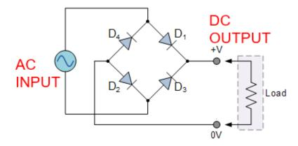
**Bridge Rectifier to CDU Wiring Diagram**: The four diodes are a standard 400Volt 1Amp IN4004 (eg. JayCar code ZR-1004) but just about and general purpose rectifier diode will do the job just fine. These diodes have a silver band on one end that corresponds to the "bar" end in the Bridge Rectifier diagram above. I have marked these with the red lines to make it more visible as it's very important to get them connected correctly. The two "bar" ends are connected to the positive input of the CDU.
