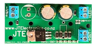
This CDU will allow switching a Point/Turnout motor without fear of burning out the motor coils if a control switch gets stuck in the "ON" position – most commonly when the switch contacts get welded together.
