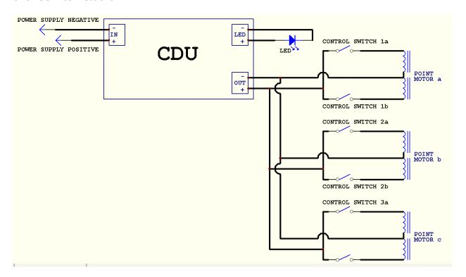
On large track layouts you may need to use heavier gauge wire on long wiring runs between the CDU, control switches, and the point motor. As an alternative, you could install another CDU on the other side of your track layout nearer to the other group of control switches and point motors so you can use shorter wiring to the second group of point motors and control switches.
