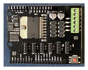
The JTEMOT1 is a standard "Arduino Motor Shield R3" with the L298HN IC in its horizontal MultiWatt15 package providing far better thermal performance than other shields that use this IC in its PowerSO20 package.
