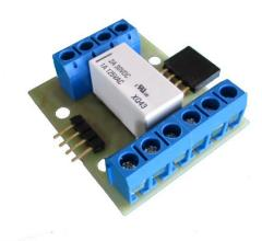
This relay board will allow switching power to tracks or points or turnouts or lights or whatever other purpose you see fit with separate control coils for "SET" and "RESET" relay states. The relay is a "latching" type meaning the output contacts will stay in either the SET or RESET position even when power is removed from the relay control coils. Its like they have a "memory".
