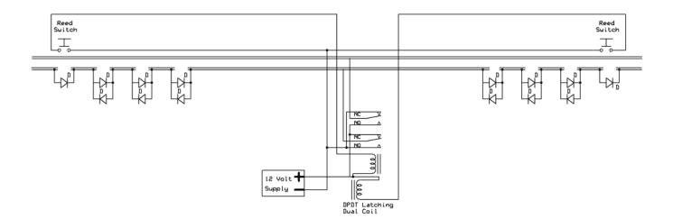
Better still, you could easily replace the reed switches (and magnets on all the first and last rolling stock) in these diagrams with my JTEILD infra-red locomotive detector boards at either end of the track to detect the train. The JTEILD boards are more reliable at detecting the train and don't require any modification to the locomotive / rolling stock / train!
