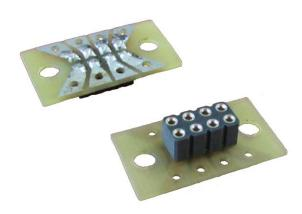
This DCC Socket Board will allow you to make a locomotive "DCC Ready" and allow plugging in a standard DCC Decoder board to control the locomotive. The eight individual pin sockets are brought out to eight larger pads on the board to allow connection of the locomotive wiring.
