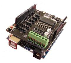
We have carefully followed various documents and videos to bring you the JTEDCC - a fully constructed and tested DCC basestation controller for a fraction of the price of commercial units. The JTEDCC module comprises of an Arduino based microcontroller shield and a motor controller shield. It connects to your computer via a USB cable and also connects to two tracks – your mainline, and a separate programming track.
