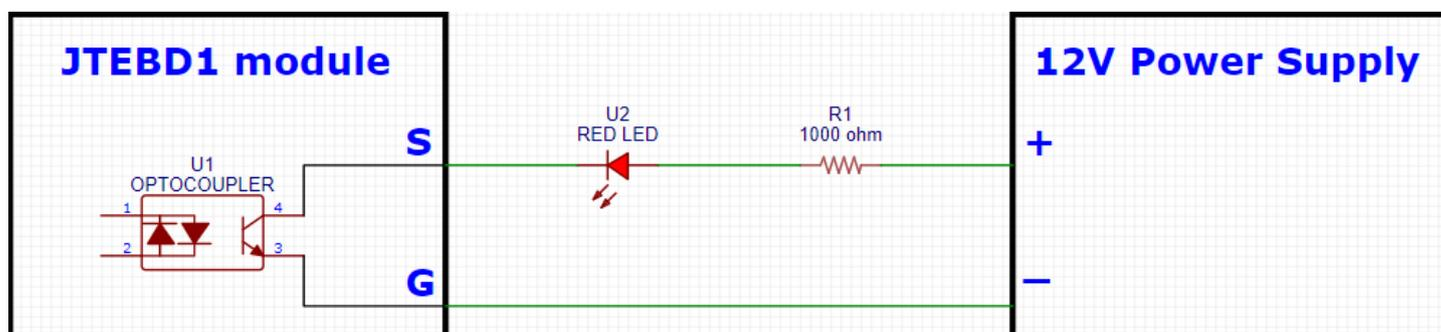
The JTEBD1 output can be directly connected to a microcontroller input pin. Don't forget to use a pullup resistor so the microcontroller sees a “HIGH” level when the JTEBD1 has not detected your train and sees a “LOW” level when your train is detected on the block of track and the optocoupler gets turned on.
